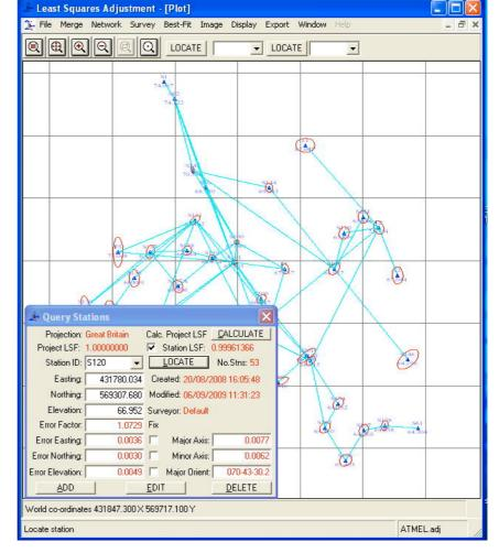
it own least squares adjustment, error propagation and analysis computer software to ensure that all the survey control networks, surveys and setting-out are precise and accurate. The error analysis confirms that the quality of the survey control network meets the specified tolerances and any subsequent survey activities can be undertaken with confidence this analysis can be delivered to the client as a stand-alone document or embedded into a drawing as text.
